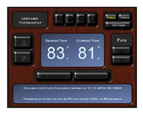
*Turning Off HOLD:* You can stop the thermostat from holding by pressing the highlighted HOLD button. Hold mode will also be stopped if a change is made at the thermostat hardware.
