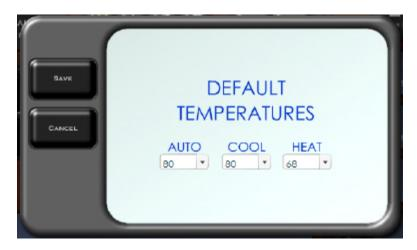
You will see a default temperature setting available for each thermostat mode. The OFF mode is not listed since the thermostat will not be running at all in that mode.
