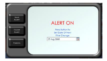
*To Clear your alert*, press the Clear Alert button under Filter options for the desired thermostat.
