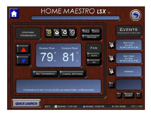
The thermostat screen has a large window in the center of the screen that will display the desired temperature and the current temperature of the selected thermostat.
